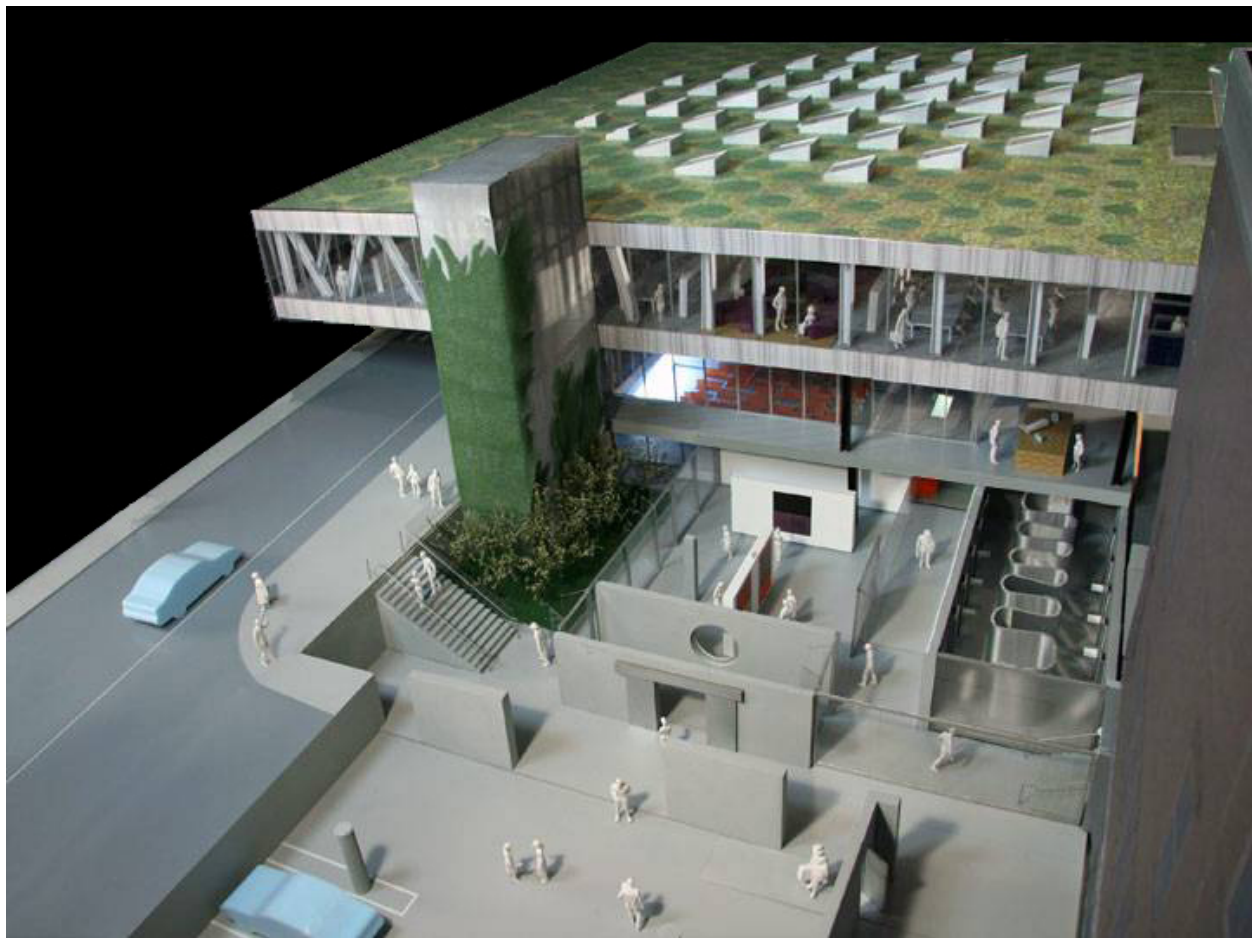
Figure 1.4.22: View of the garage interface. The surface level has been removed in this image to show the lower-level connections below grade.
