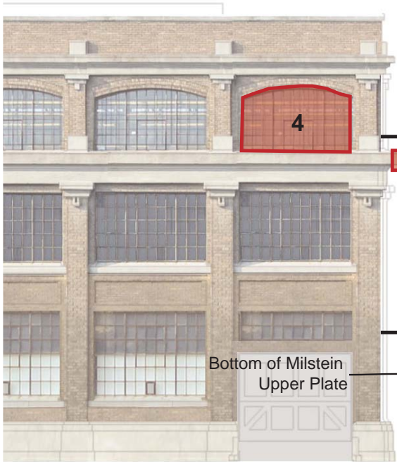
Rand Hall: Removals at North Wall
